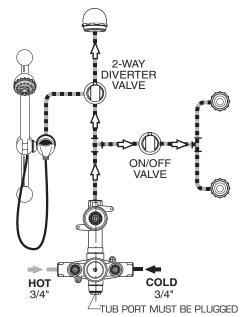
**NOTE**: MINIMUM FLOWING PRESSURE REQUIRED FOR THIS SYSTEM OPERATING WITH ONE SHOWER HEAD AND 2 BODY SPRAYS IS 40 PSI
